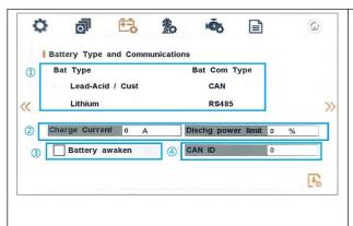
①Set Battery Type and Battery Communication method.
