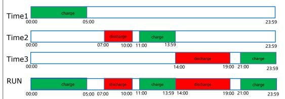
3) If you want to set a continuous charging time from the first night to the next morning. For example, you want to charge the battery from the first day 21:00pm to the next day 5:00am, divide this time period into two time periods  $(21:00\sim23:59,\ 00:00\sim05:00)$ , and select two charging time periods from Time1, Time2 and Time3 and set them.
