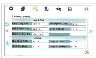
①Settings required when using lead-acid batteries
