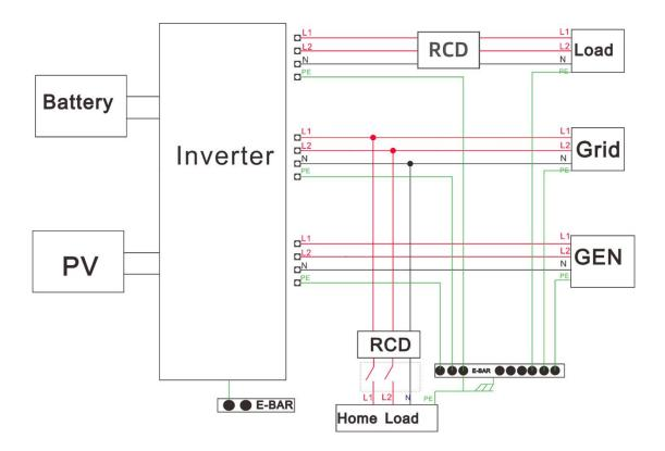
All switches and RCD devices in the figure are for reference only, and the specific installation shall be subject to local regulations.
