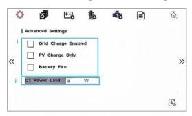
**i.** Users have three advanced settings to choose from, namely Global Grid Charge Enable, PV Charge Only and Battery First.
