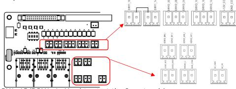
DRY1\_1B/DRY1\_1: Used to start the Inverter driver.
