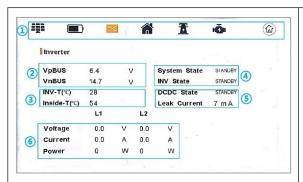
①Users can click on the icon above to switch device status data (PV, Battery,
