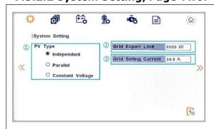
① Users can set PV types, including Independent, Parallel and Constant Voltage.
